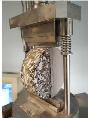
Figure 7. ITS set up for MMT sample.
